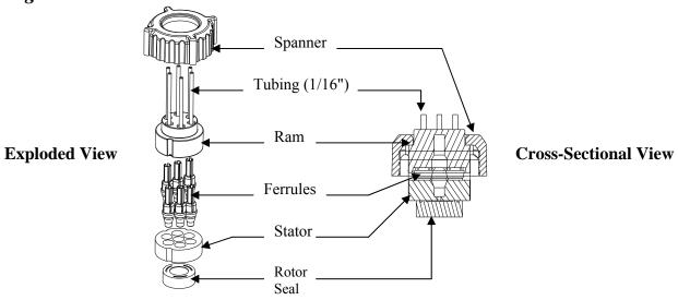
\* This model includes 1/16" O-rings at the base of the stator ports. These must be removed for use with 1/8" ferrules and tubing.
